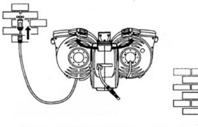
3. To release, pull the hose away from the reel. You will feel the hose start to rewind, walk back with the hose towards the reel. Do not simply let go of the hose (see pic).
