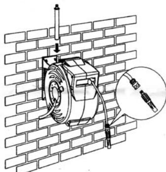
4. Attach the 2m tap to reel connector to your tap using the universal tap adaptor. Test to ensure the reel rotates freely though 180° with the tap adaptor connected.
