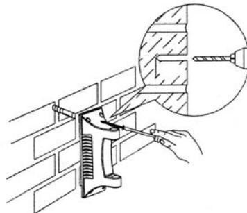
3. Align the back of the reel with the wall bracket and insert the securing pin through the join.
